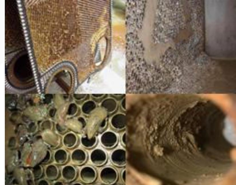
Figura 15: Fouling, Fuente: Heat Exchanger Fouling: Mitigation and Cleaning Techniques
